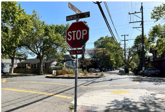
Left: Ninth Street and Allston Way intersection with traffic circle. Drivers approaching the intersection were seen encroaching on the curb as they made wider-than-necessary turns around the traffic circle.
