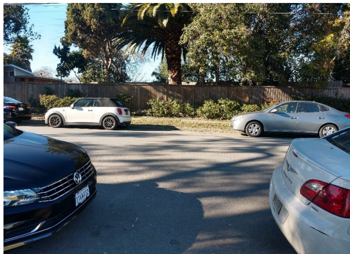
Above: Unevenly spaced car parking limits curb capacity.
